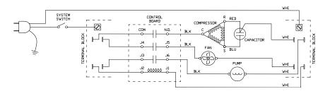
GEYSER Internal Wiring Diagram
