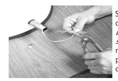
Squeeze the "UR" connector with a pair of pliers, or tap gently with a hammer. *Do not use unneccessary force when squeezing the red "UR" connector.* The red "button" on the connector will be pressed in until it is even with the top of the connector.
