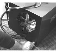
Now, completely open the valve *closest* to the tank and check for leaks. Then *slightly* loosen the hose connection at the valve furthest from the tank to allow air to breathe. You may possibly hear some air evacuate and/or have a few drops of water emerge from the connection. Once done, retighten hose connection, and open the valve completely.
